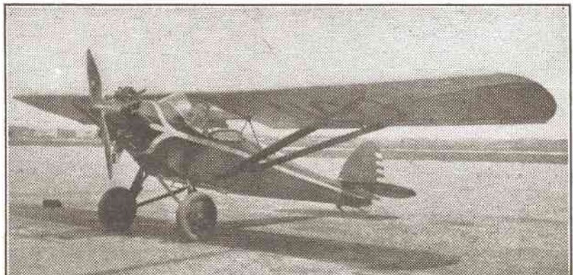
For the sport flyer who wants an open cockpit job, we highly recommend the Monosport, the open-cockpit version of the reliable Monocoupe. This ship, powered by the 125-h.p. Warner radial engine, is one of the best bets for its weight in the country.
