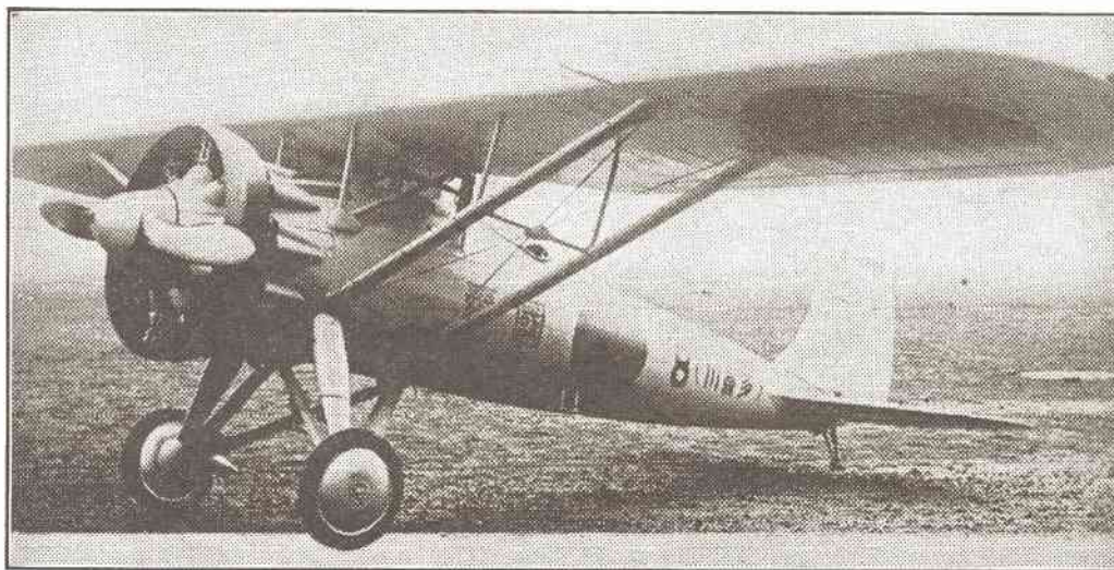
This single-seat Nakajima 91 fighter has long been a favorite with Japanese army flyers. A French-type monoplane, it carries two Vickers and travels in the neighborhood of 200 m.p.h.
