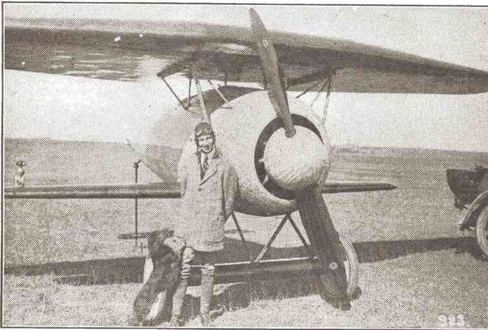
Left: From the Nioto Collection comes this fine photo showing Tony Fokker at the height of his war-time designing career before his first cantilever winged plane, the V-1. Note the stub section, airplane airfoil and the unusual aneroidometer fitted near its right tip. On this job, Fokker used the Oberursel rotary engine, a copy of France's famed LeRhone. But though her trimness is undoubted, we have been unable to find any record indicating that this plane was ever used by the Boches in actual war service. The Germans, it seems, were afraid of the cantilever wing idea until it was later proved feasible beyond doubt in Fokker's renowned D-8 model. A mighty speedy cooling bus, though, this V-1!
