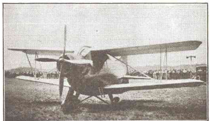
This Gwinn Aircar, which was on view at the Races, is the ship which made Frank Hawks forget his "Time Flies." Featuring a tricycle landing gear, it's designed for family use. Hawks will be busy demonstrating it for quite a while.
